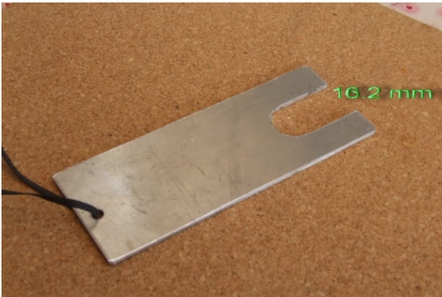
Image 2a (Home made separating tool for Hydraulic Pipe Connector)
